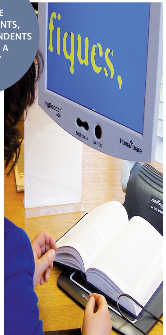
Innovative myReader system that allows visually impaired users to read for long periods without feeling sick or tired
